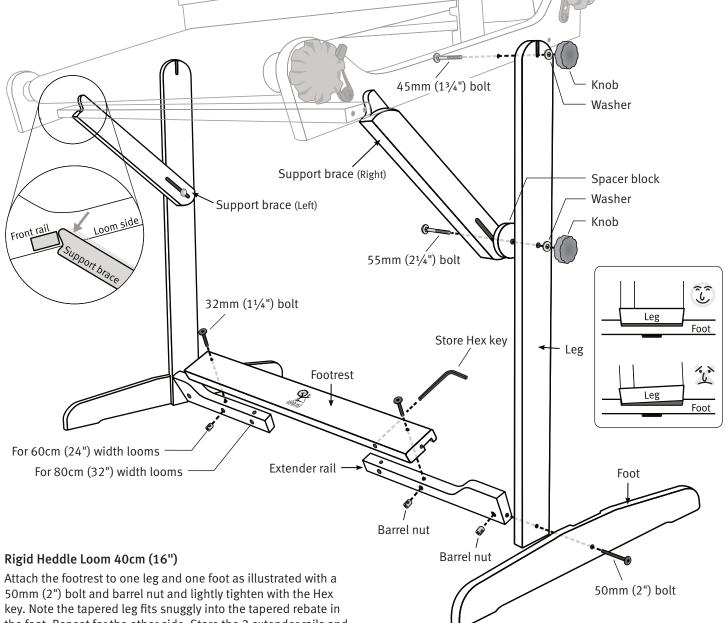
the foot. Repeat for the other side. Store the 2 extender rails and 32mm (11/4") bolts and barrel nuts for future use with either a 60cm (24") or 80cm (32") Rigid Heddle Loom. Proceed to Step 3.
