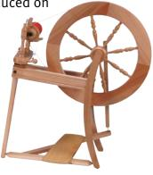
1989 - Three speed flyer. Treadle board supplied assembled onto the treadle rails. Single bolt and barrel nuts used to assemble frame. Leather conrod joint replaced with round polyurethane connector.
