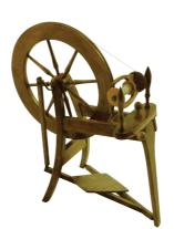
1981 - Two speed flyer with click-fit flyer bearings allow the bobbins to be changed without turning the maid upright. Tension knob is located on the front of the maiden bar to be closer to the spinner. The crank is now one piece with a cotter pin securing the con rod in place. The wheel is finger-jointed for extra strength.
