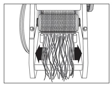
**Prepared fibre** - Peel sliver into strips, stretch to lengthen and spread it out sideways. Place on the feed-in tray and turn handle clockwise. Allow the fibres to feed-in, don't hold back.
