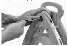
**2.** Remove the four screws that retain the back frame to the four dowel spacers.
