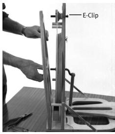
7. Place the drive belt around the wheel and pulley. Then replace the back frame into position carefully sliding the flyer and crank back through the ball bearings. **Note:** Take care not to push the ball bearings out of the plastic bearing housings.
