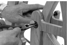
**9.** Replace the screws holding the back frame to the base and dowel spacers.
