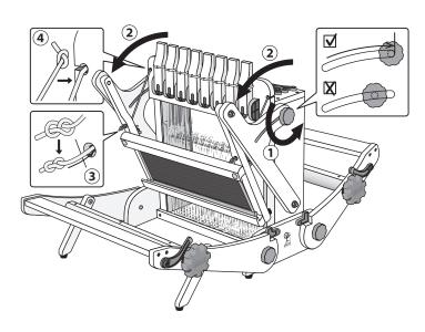
**Step 6:** Push the levers down and check the gap between the shafts and the castle top is approx.  $1 \text{cm} (\frac{1}{2} \text{ins})$  on both sides. Adjust the height as necessary by moving the Texsolv cord in the lever or on the screw head in the shaft end.
