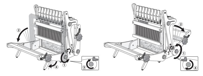
**Step 4:** Loosen knobs securing the beater supports, slide the beater completely forward and tighten the knobs.
