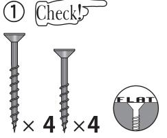
Attach the castle top to the castle sides with  $4 \times 38 \text{mm} (1\frac{1}{2})$  screws. Check that the pilot holes for the castle front are all on the same side.
