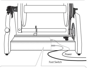
NOTE: ensure the e-Spinner Super Jumbo is switched OFF before removing the foot switch plug.
