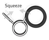
**5.** Locate the drive band onto the MIDDLE groove in the bobbin whorl. Do not use the large groove as this will stretch the drive band. We have used the Country Spinner2 Bobbin as standard on the e-Spinner Super Jumbo, so they are interchangeable between the two spinning wheels.
