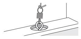
**4.** Thread the screw eye into the pilot hole in the right-hand side.
