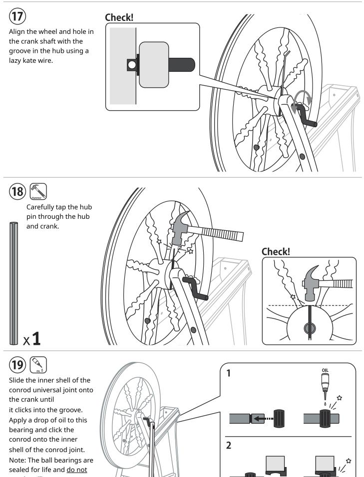
Note: The ball bearings are sealed for life and <u>do not</u> require oiling.
