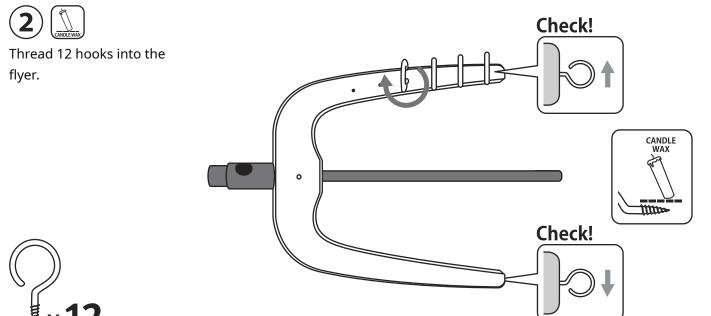
Assemble the flyer unit. Check the shape of the nylon bearing on each maid upright, wax the dowel ends, then insert into the correct hole. Insert the drive belt
