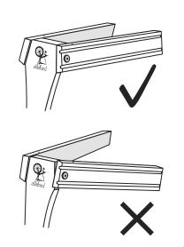
(11)Check! Set the treadle assembly on the edge of a table. Insert the conrod joint into the large slot in the treadle rail. Note the crank bearing faces the back of the spinning wheel. 1. Hold the conrod joint with one hand on either side of the treadle rail. 2. With both hands, turn the conrod joint a ¼ turn, 3. stretch and slide it into the small slot and turn it back a ¼ turn until it clicks into place.
