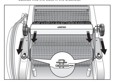
5. Rotate the packer brush until the bristles are about  $\frac{1}{2}$  way into the carder teeth, then tighten the 2 knobs.
